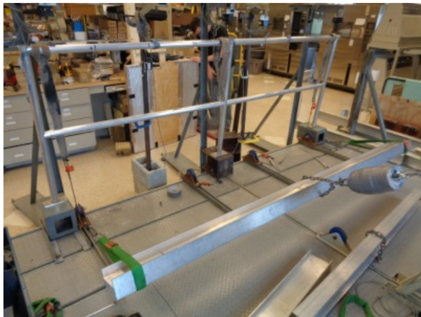
Photo No. 6 Vertical Concentrated Load on Top Rail Adjacent to End Post
