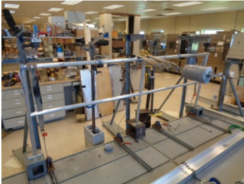
Photo No. 7 Concentrated Horizontal Load at Top of Post
