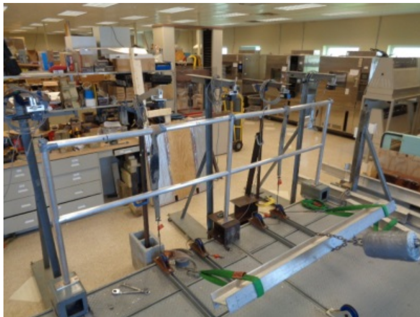
Photo No. 4 Vertical Concentrated Load at Mid-Span of Top Rail
