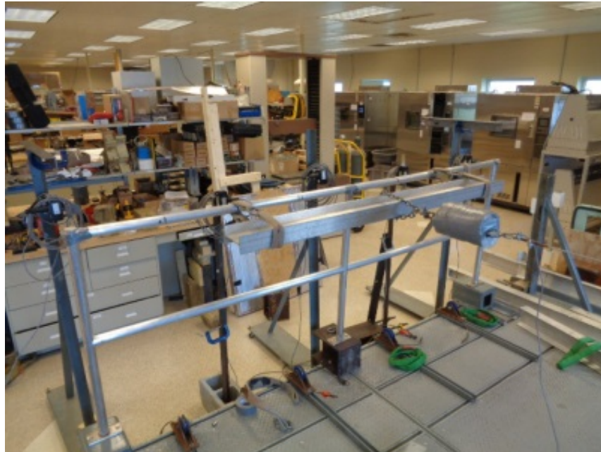
Photo No. 3 Horizontal Concentrated Load at Mid-Span of Top Rail
